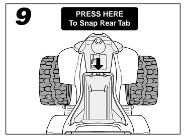
Press firmly on the back of the cowling to snap the rear tab into the slots in the vehicle body.
